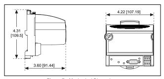
Figure 7. Mechanical Dimensions
